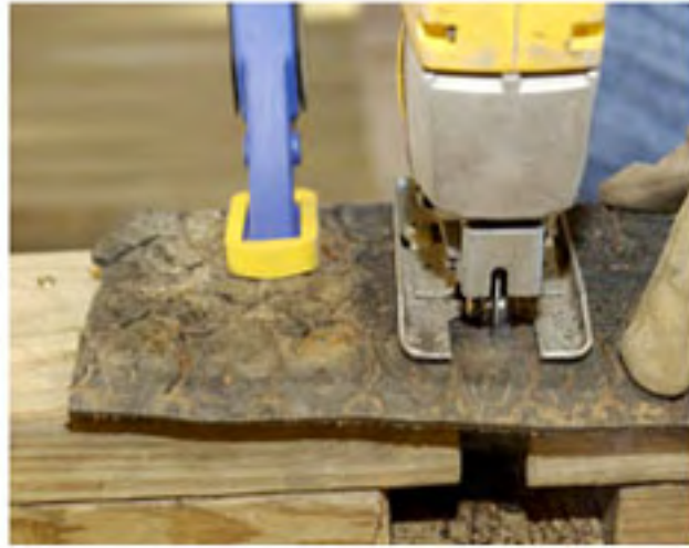
Using a jigsaw to cut through tire tread.
