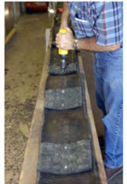
A simple elevated workbench for extra long rubber boards.
