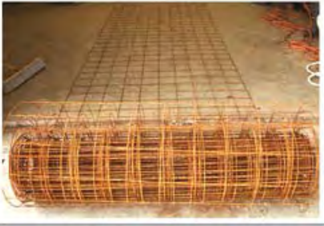
A roll of concrete reinforcing mesh
