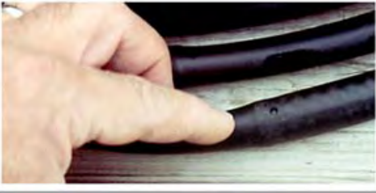
A hard hose emitter line with a dripper (hole) visible
