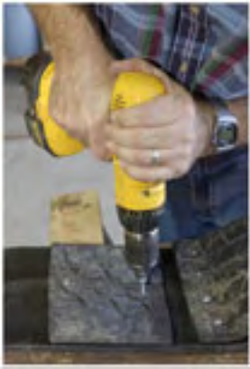
Fastening a 6-inch wide piece of rubber to the board to form a pocket.
