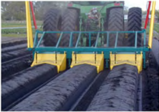
Temporary raised beds made with a tractor and a bed shaper.
