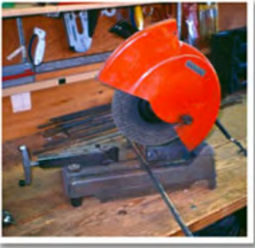
Use of a chop saw to make rebar stakes
