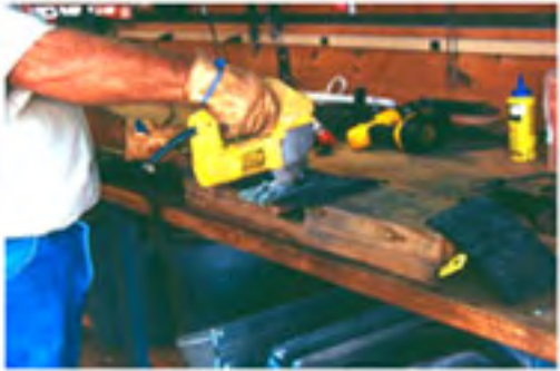
Sectioning tread with a cutting jig made from three laminated 2- by 12-inch boards. A gap between the top two boards is necessary to provide clearance for the blade.
