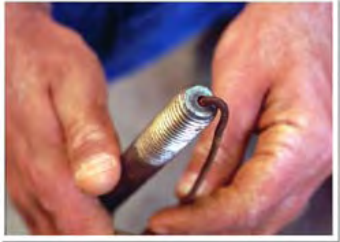
Using a bolt to bend wire "fingers"
