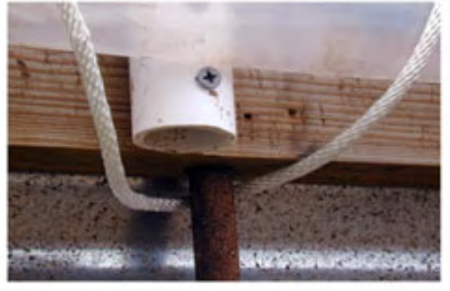
Proper orientation of hold down rope strap at point of attachment to bed
