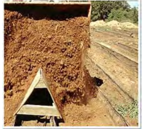
A soil portioning tool, when used with a front-end loader, directs soil into the beds, saving time and energy during bed filling.
