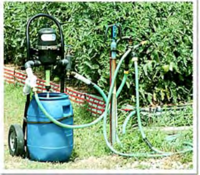
A fertilizer injector makes "fertigation" (the application of fertilizer through the drip system) possible.
