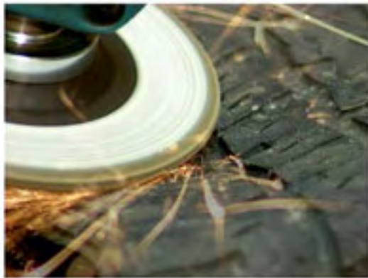
Removing screw tips with a grinder.
