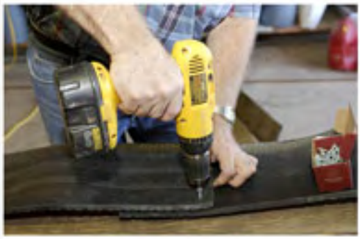
Fastening one piece of tread to another. Orient pieces with tread facing down.
