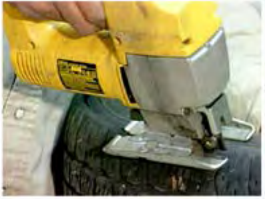
Use a jigsaw to remove sidewalls from the tires.
