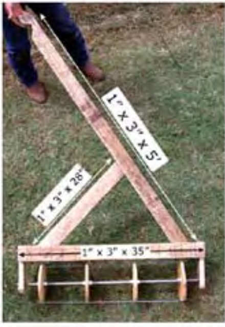
Dimensions of the Noble Foundation rolling row marker the face of the axle body.
