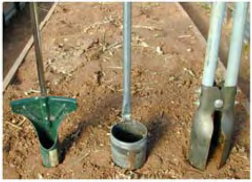
Tools for digging transplant holes: left, a bulb planter; middle, a customized soil extractor made from electrical conduit and thin-walled pipe; right, a post hole digger
