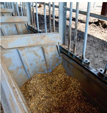
In the GrowSafe system, RFID antennas are molded into the rim of each trough. The trough is suspended on parallel load cells that weigh the trough to a resolution of 10 grams. The system continuously scans the feed bunks, recording feed disappearance and accurately identifies the animal's location, feeding behavior and feed intake.
