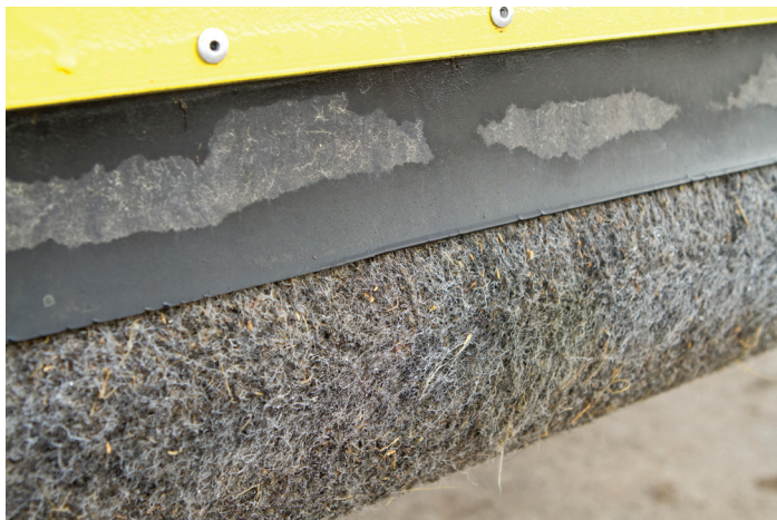
The spray boom, which wets the carpet-like wiping surface on a rotating-type wiper, is enclosed by the black and yellow shield
