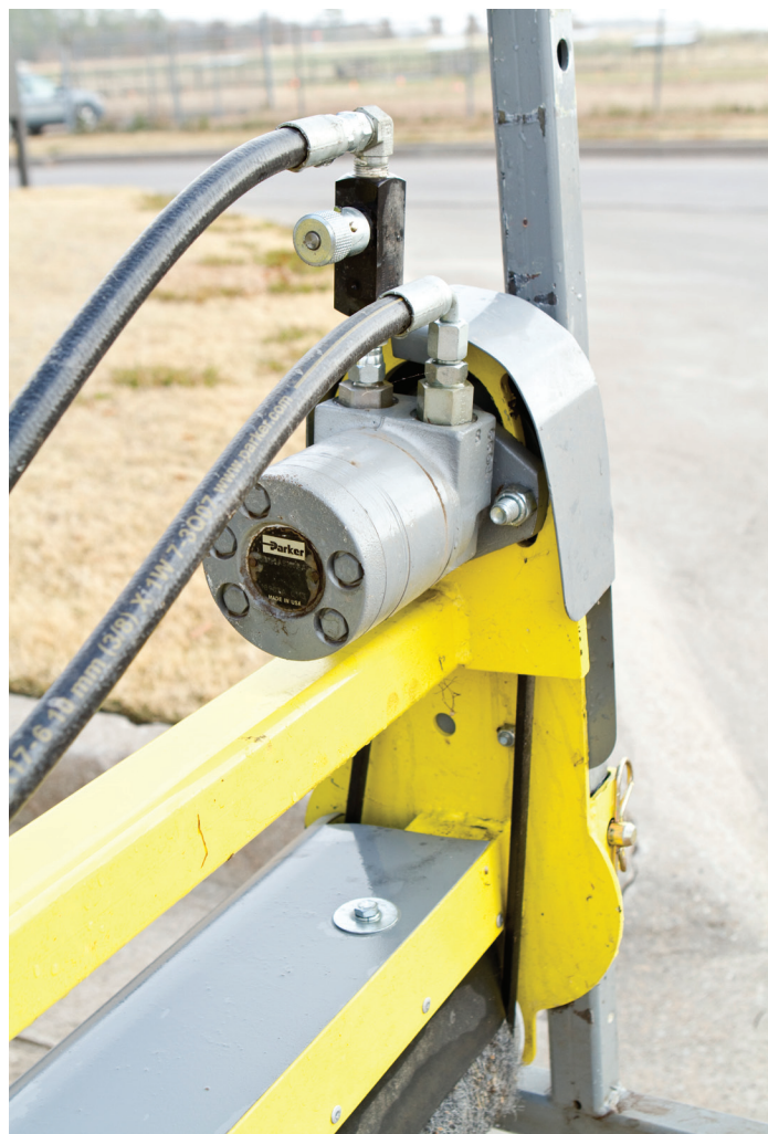
A hydraulic motor counter rotates the wiping surface on this rotating-type wiper. Some units use a ground drive wheel instead of a motor.
