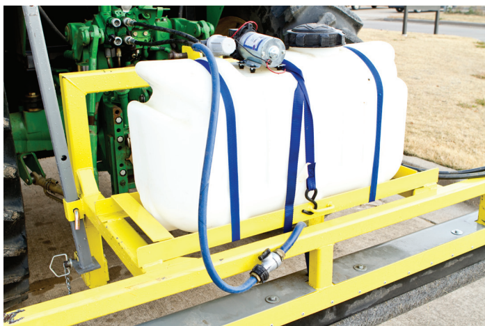
Small 12-volt pump on rotating type wiper
