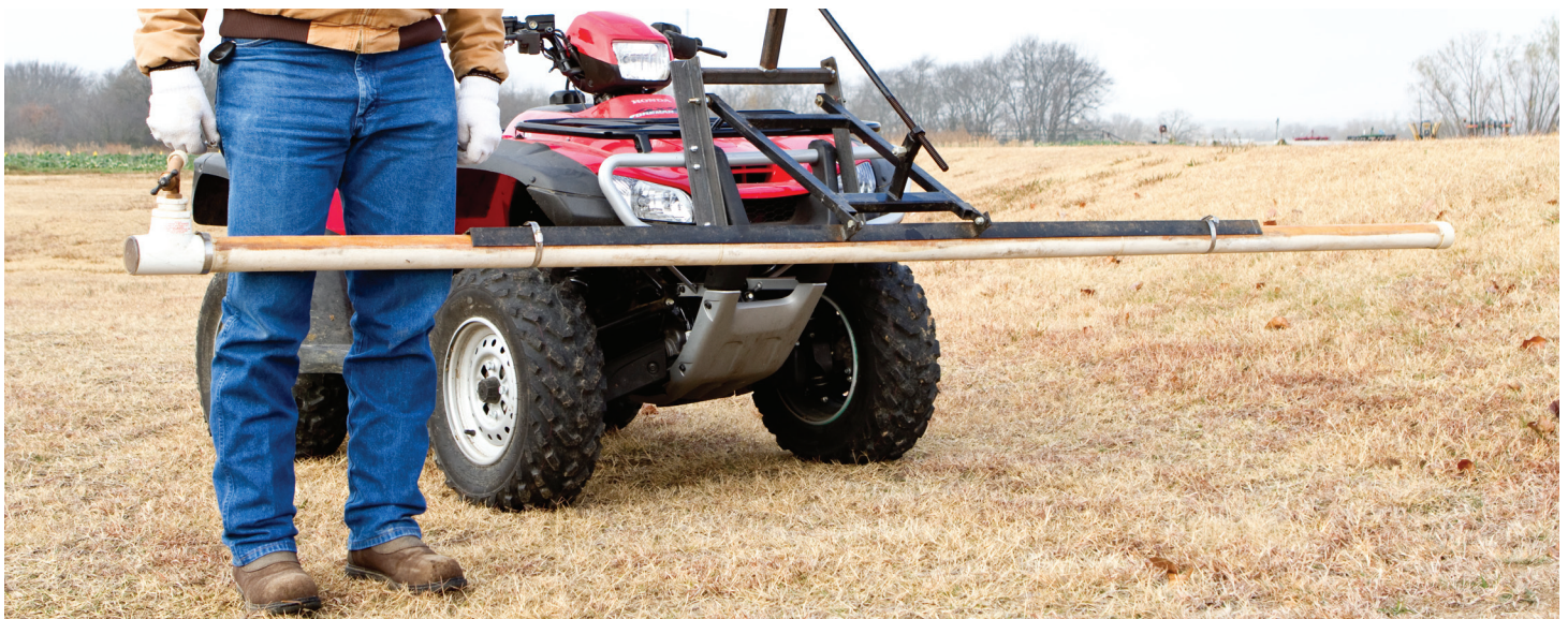
Notice difference in height from side to side on sloping terrain
