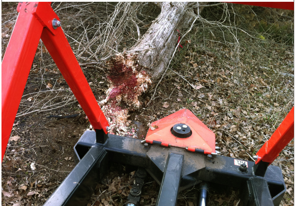
Close-up of tree saw mounted on the front of a skid loader
