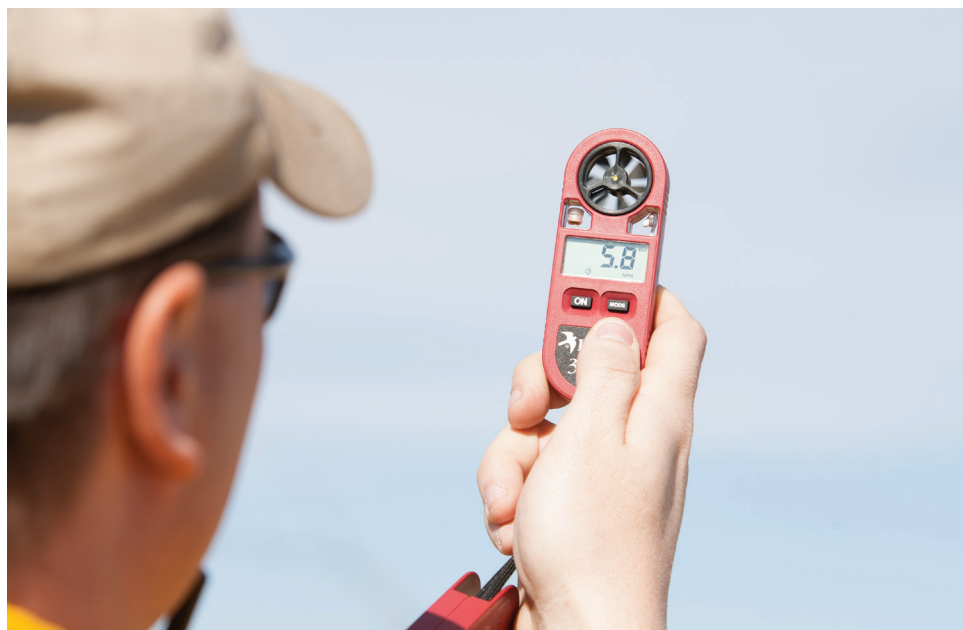
A Kestrel Weather Meter is used to monitor on-site weather during a prescribed burn.
